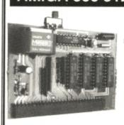
Direct replacement for the A501 Expansion • Convenient On/Off RAM Switch . Autorecharging battery-backed Real-Time Clock •
